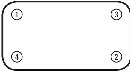
Tighten all screws to an 8 inch-pound torque. There may appear to be a gap between the lid and the base. This is normal. Over-tightening of screws to close the gap is not recommended.
