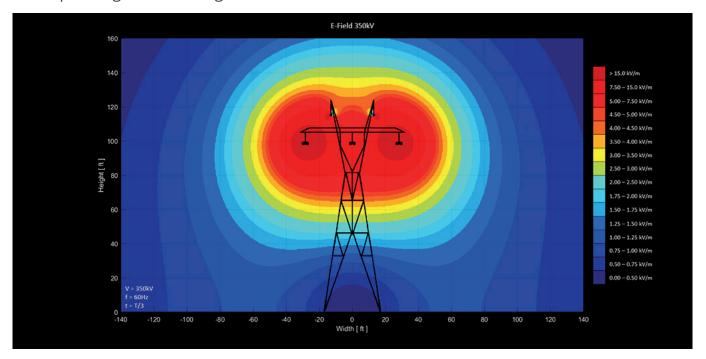
Proximity alarms detect E-fields, not OSHA distance regulations, that can change and vary depending on the equipment being operated and other factors. OSHA requires the employer to identify the safe distance.
