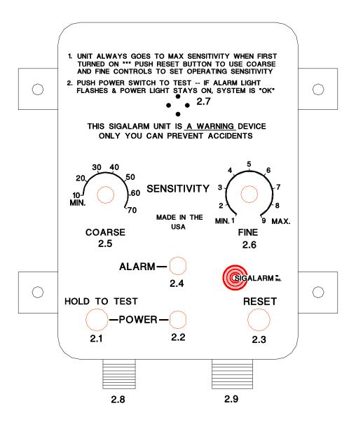
**2.1 HOLD TO TEST BUTTON** - allows the operator to test the entire system by pushing and holding down this button. This button then checks the entire system, if the green power light stays on, external horn sounds, internal buzzer works, and red light flashes the system is fully functional. If any of these are not working contact your supervisor and fix prior to use. If any of these fail there is either a break in the antenna, a jumper pin problem, or there is an internal failure.
