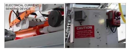
Photos 8 and 9. Example of proximity warning device used on aerial ladder truck at neighboring fire department. Photos left to right – electrical current sensing device, and alarm and control box. (Photographs courtesy of neighboring fire department.)
