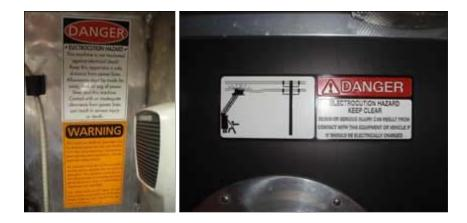
Photos 3 and 4. Shown here are two of the four warning signs affixed to Truck 2.
