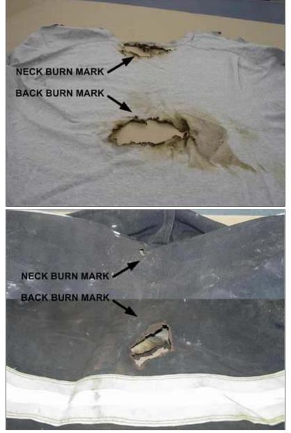
Photos 5 and 6. Victim's T-shirt and bunker jacket with burn marks on the neck and back area from contact with the energized electrical powerline. (*NIOSH photographs.*)
